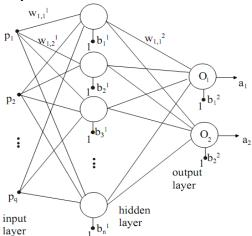
Fig: 3. Multilayer Feed-forward Neural Network
