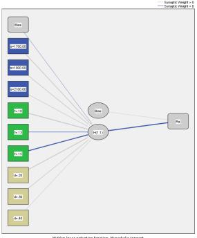
Hidden layer activation function: Hyperbolic tangent Output layer activation function: Identity
